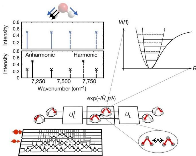
**Figure 5: Quantum photonic integrated circuit with thermo-optic phase shifters (bottom) allows for simulating the vibrational quantum dynamics of molecules (taken from Nature (2018): <https://doi.org/10.1038/s41586-018-0152-9>)**
