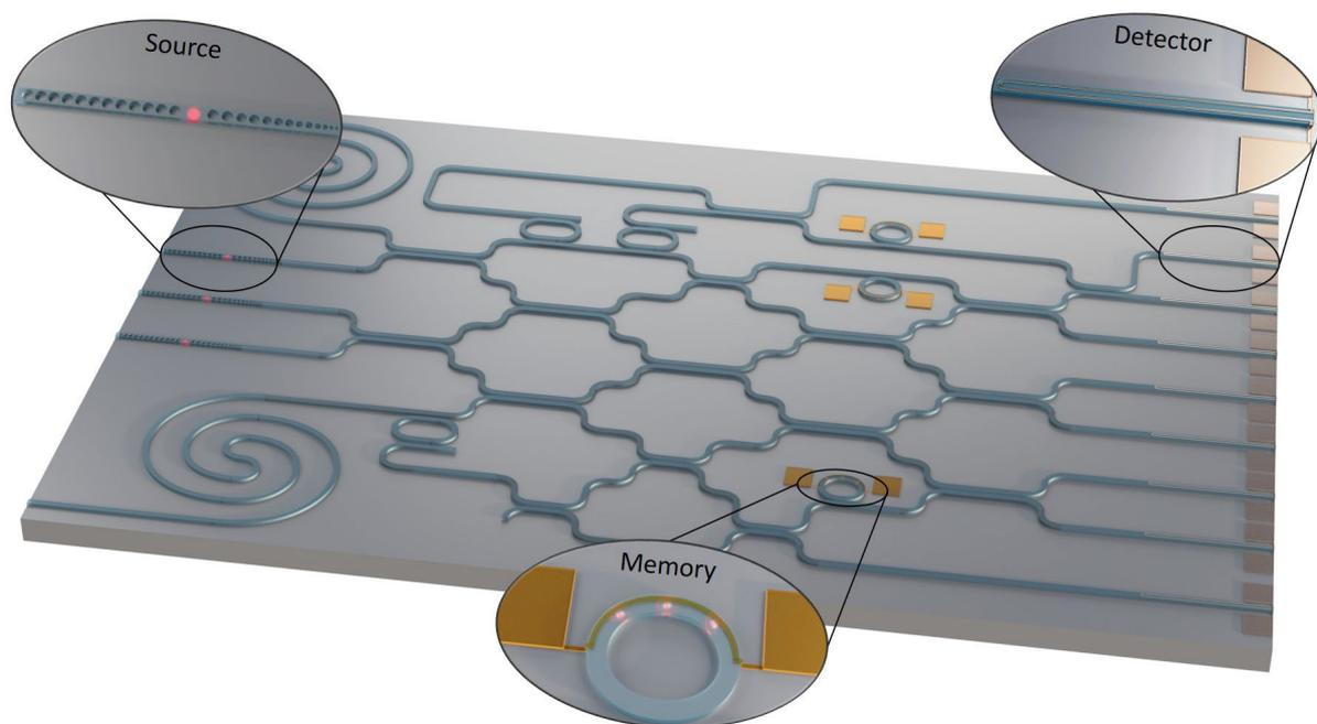
**Figure 1: Quantum photonic integrated circuit, including non-linear optics (spirals) and quantum light sources (red dots) in nano-beam cavities, quantum memories (rings including ions), and superconducting detectors (strips), as well as active and passive photonic elements (taken from Nat Rev Phys (2021): <https://doi.org/10.1038/s42254-021-00398-z>)**
