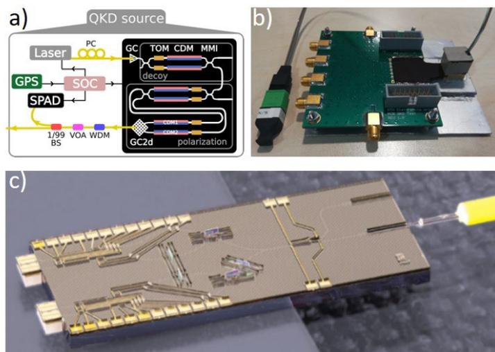
Figure 2: a) shows the scheme of the QKD state generator system and b) the integrated chip including connectors (taken from Quantum Physics (2019): <https://doi.org/10.48550/arXiv.1907.10039>) . c) Photonic circuit with hybrid integration of transceivers for CV- and DV-QKD, including InP based single photon detectors (courtesy of HHI)
