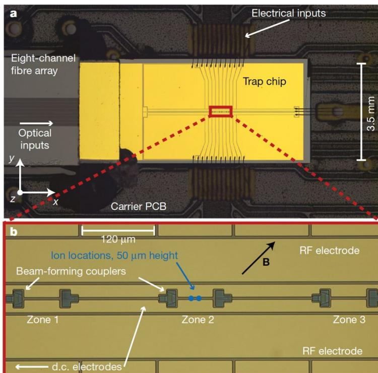
**Fig. 4: Optical micrograph of an assembled ion trap device with an eight-channel fibre array attached. b, Higher-magnification view near the trap zones (taken from Nature (2020) <https://doi.org/10.1038/s41586-020-2823-6>)**
