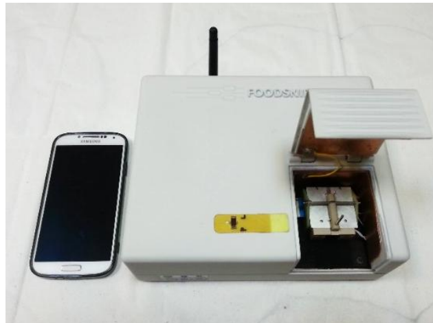
Photograph of the FOODSNIFFER system where one can appreciate its compact size compared to a smartphone. The yellow component is a cartridge with a mounted chip.
